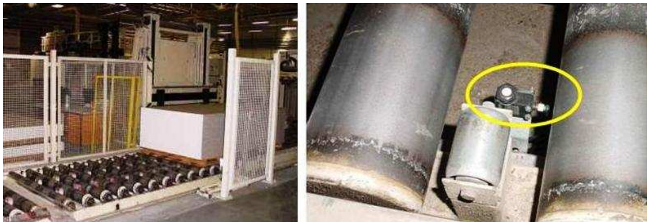
UPX ultrasonic sensor between the transport rolls
