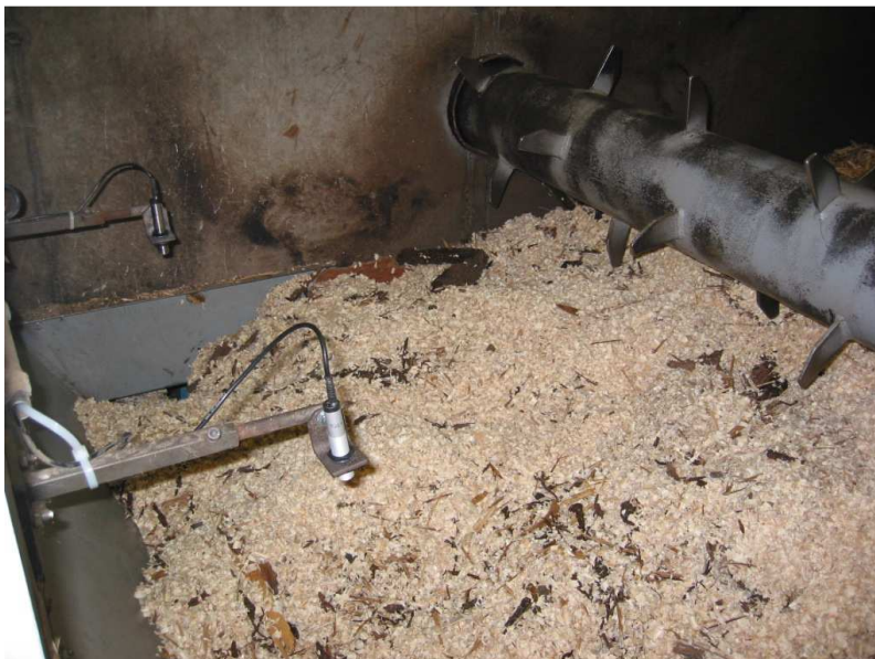
2 ultrasonic sensors above a wood chip conveyor
